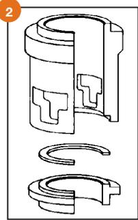
**Figure 2. Soft-Seat Ring and Ported Cage**
