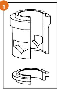
**Figure 1. Metal Seat Ring and Ported Cage**
