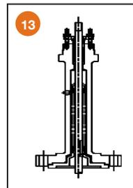
**Figure 13. Bellows Seal Bonnets**
