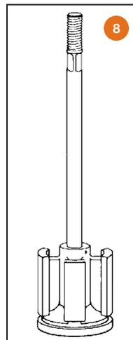
**Figure 8. Unbalanced Plug**
