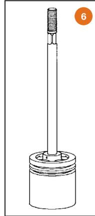
**Figure 6. Standard Balanced Plug**
