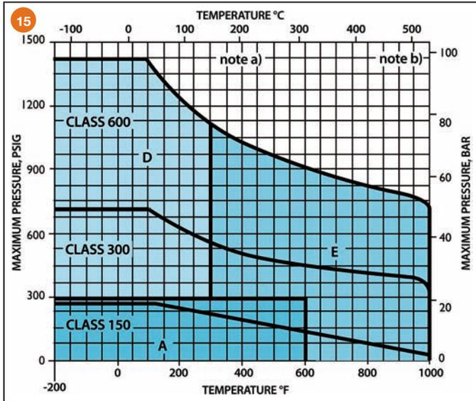
**Figure 16. Trim Chart for Carbon Steel Body (ASTM A216, WCB)**
